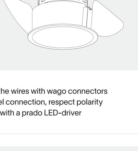
connect the wires with wago connectors for parallel connection, respect polarity
