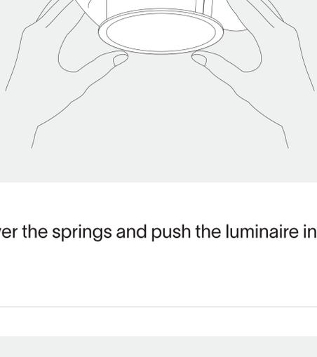
bend over the springs and push the luminaire into the ceiling
