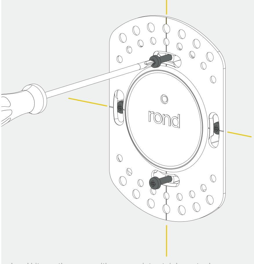
level kit, gently screw with appropriate stainless steel screws
