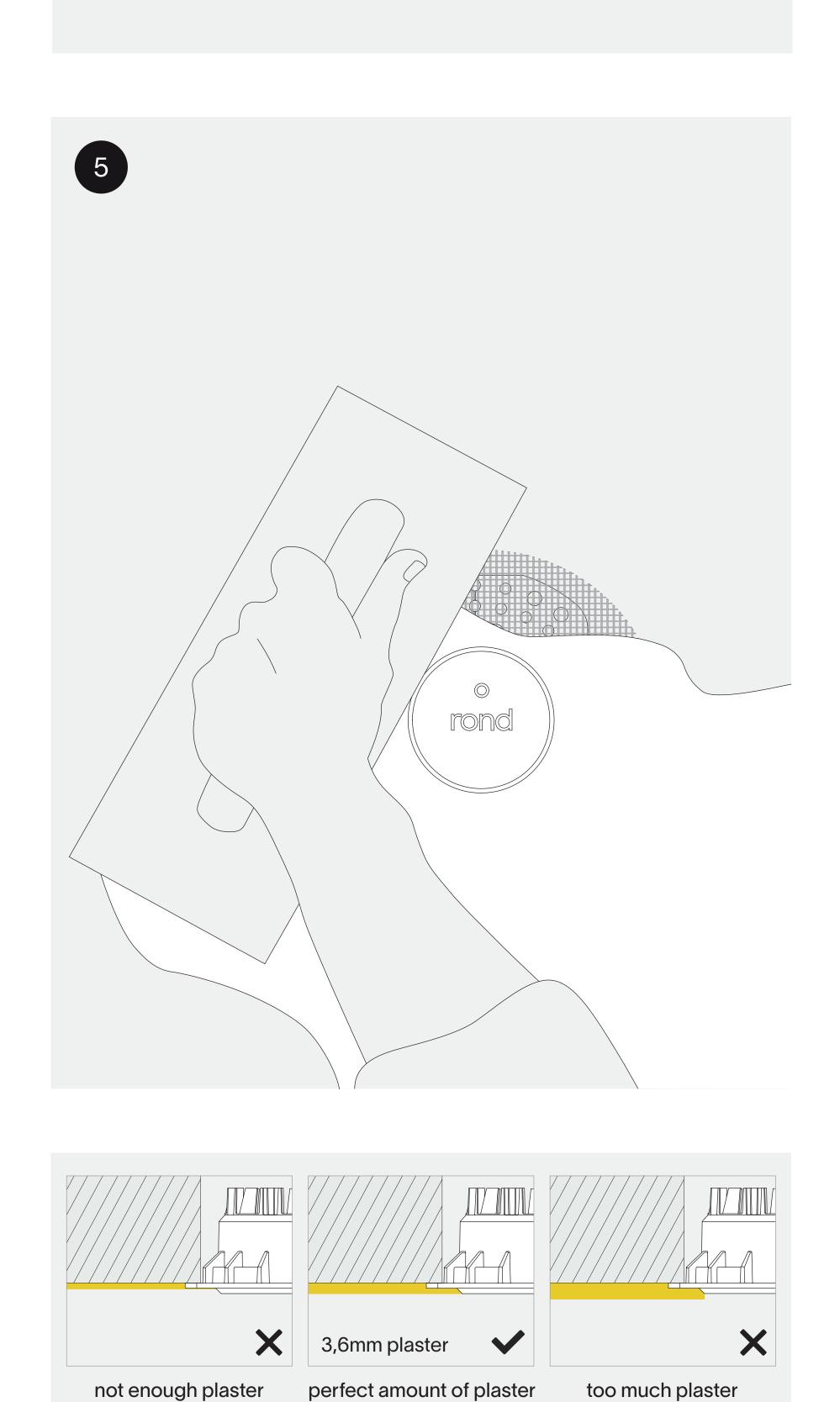
Excercise caution while plasering, do not damage the ring. Keep the plaster lid inside the plaster ring while plastering. Use a fiberglass mesh tape for optimal plaster adhesion. Make sure not to touch the edge of the ring when sanding.
