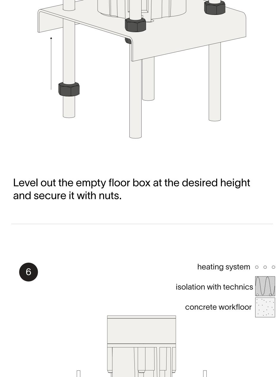
Build up all floor layers except the final concrete layer. Continue installation with the floor box Ø60 installation
