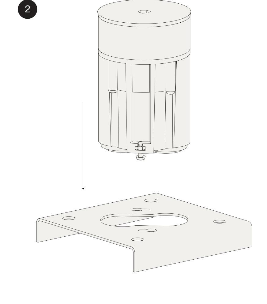
Install the empty floor box on the level support kit.
